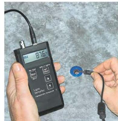
Ligno-VersaTec measuring the moisture in concrete with embedded RH BluePeg sensor
