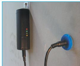
Checking drying progress behind walls. Monitor a repaired leak repair. Notice critical conditions before damage to the building structure occurs.
