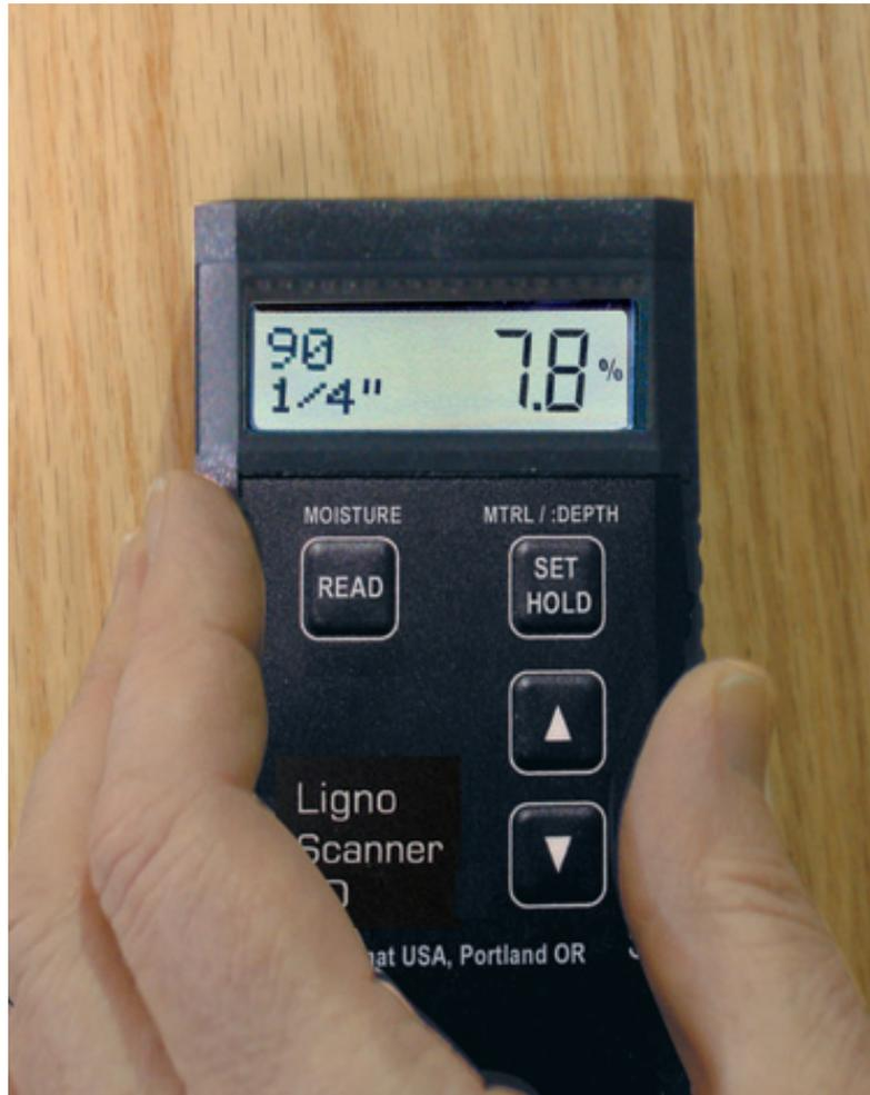
While measuring, you can toggle between the two measuring depths. Push the ▼ key to switch to 1/4" (20mm). Push the ▲ key to switch to 3/4" (7mm). One hand can hold the meter, the other hand can activate the up or down key. You do not have to move the meter at all.
