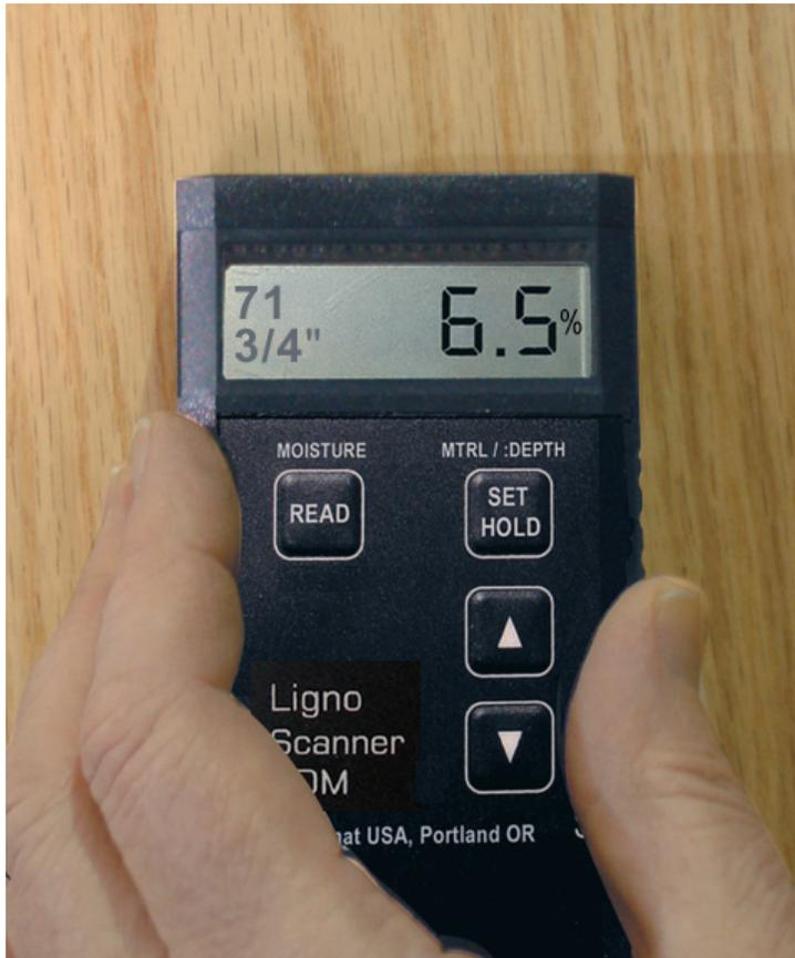
While measuring, you can toggle between the two measuring depths. Push the ▼ key to switch to 1/4" (20mm). Push the ▲ key to switch to 3/4" (7mm). One hand can hold the meter, the other hand can activate the up or down key. You do not have to move the meter at all.
