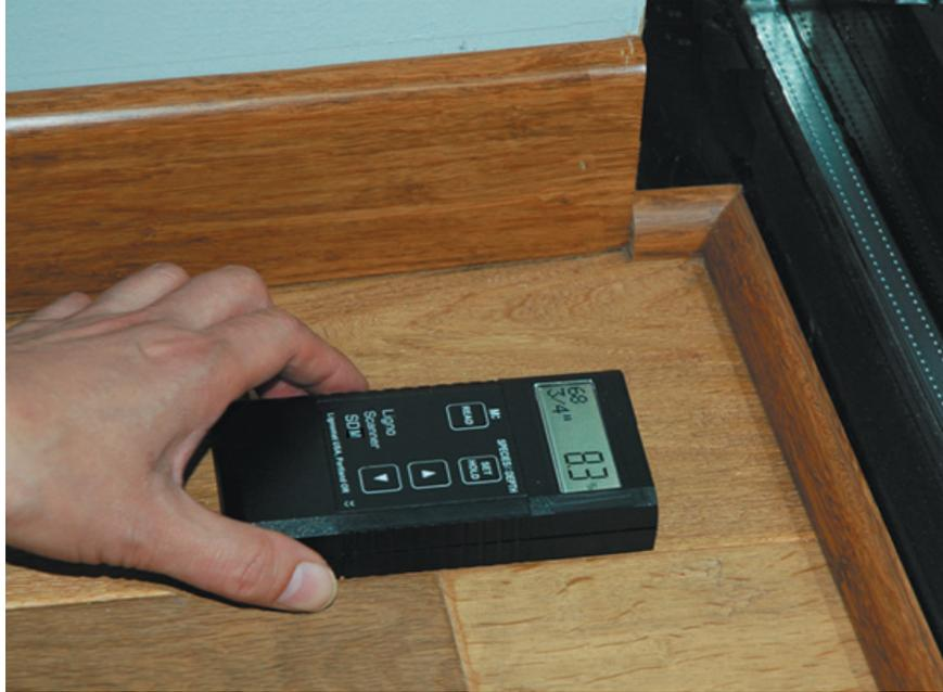
Comparing readings taken at 1/4” and 3/4” can also help to diagnose problems and indicate if moisture was absorbed from the down-side or the up-side of the floor.
