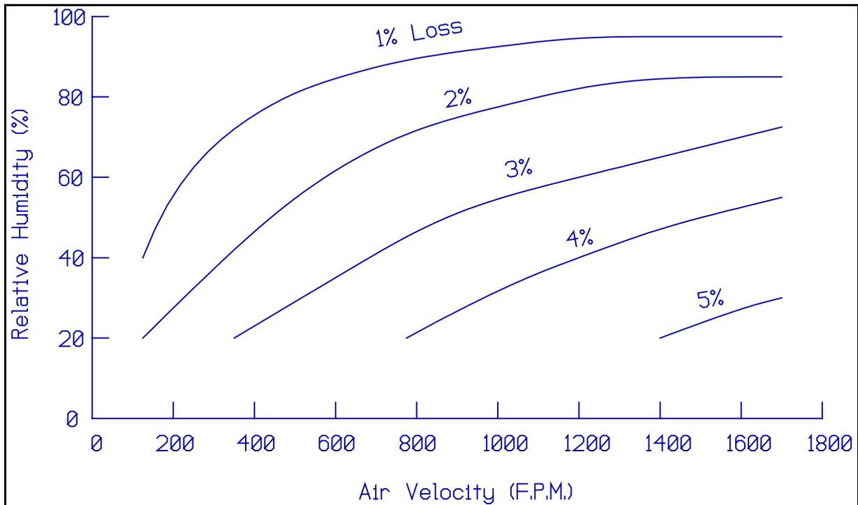
**Figure 1** Effect of Velocity on Drying Rate at Different MCs
