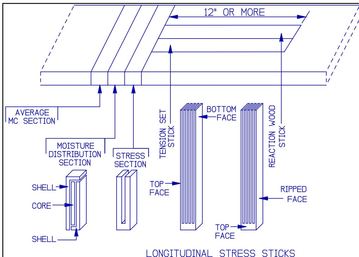
**Figure 4** Final Moisture Content and Stress Tests
